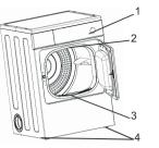
Control Panel 2.Drum Liaht 3.Filter 4.Adiustable Feet 5.Thermostat reset button 6.Side Vent offutlet 7.Vent Pipe Cover B.Rear Vent offutlet
